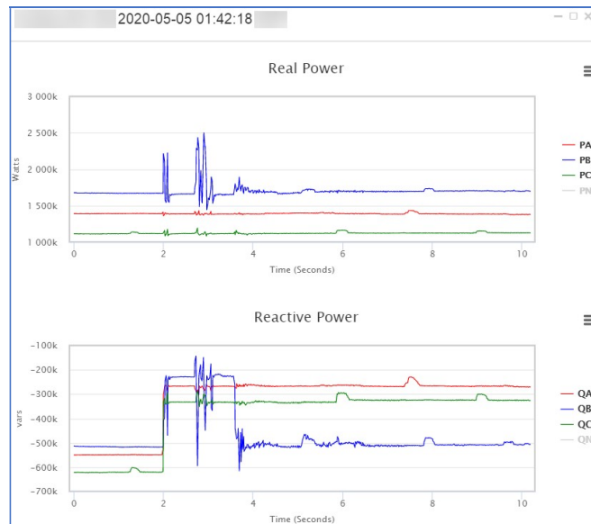
Figure 4: Real and reactive power from vacuum switch failure
